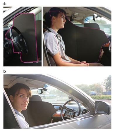
Fig. 5 (a) The Driving Wizard partition, as viewed from the driver's side (on the *left*), and passenger's side (on the *right*). (b) The participant's portion of the vehicle interior includes non-functional steering wheel, tablet interface, and video camera for recording gestural and facial reactions
