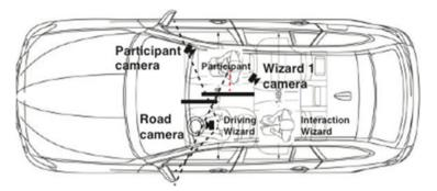
Fig. 4 The RRADS platform vehicle, noting placement of the Driving and Interaction Wizards, study participant, recording cameras, and opaque partition
