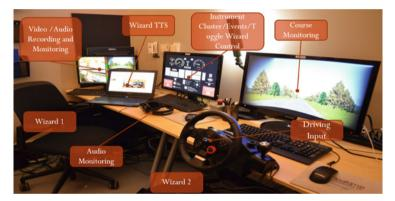
Fig. 2 The Wizard of Oz control station. Wizard 1 (the Interaction Wizard) interacts with the participant, while Wizard 2 (the Driving Wizard) initiates transfers of control and operates the vehicle during autonomous driving mode
