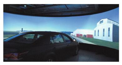
Fig. 1 The simulator used for experiments in autonomous vehicle driving and control. Participants sit in a fixed-base car surrounded by a  $270^{\circ}$  screen depicting the study environment
