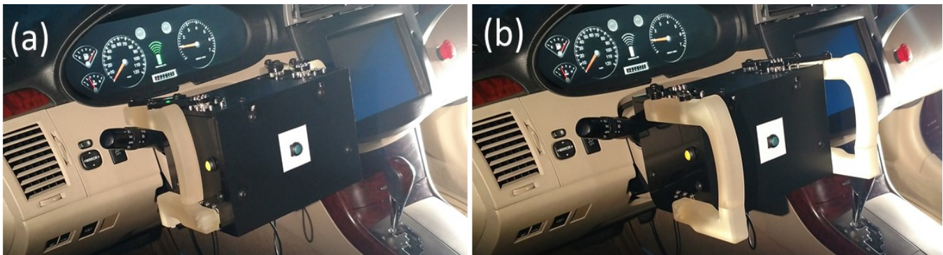
Figure 4: Final Transforming Steering Wheel Mounted in Driving Simulator. Retracted (a) and Deployed (b)
