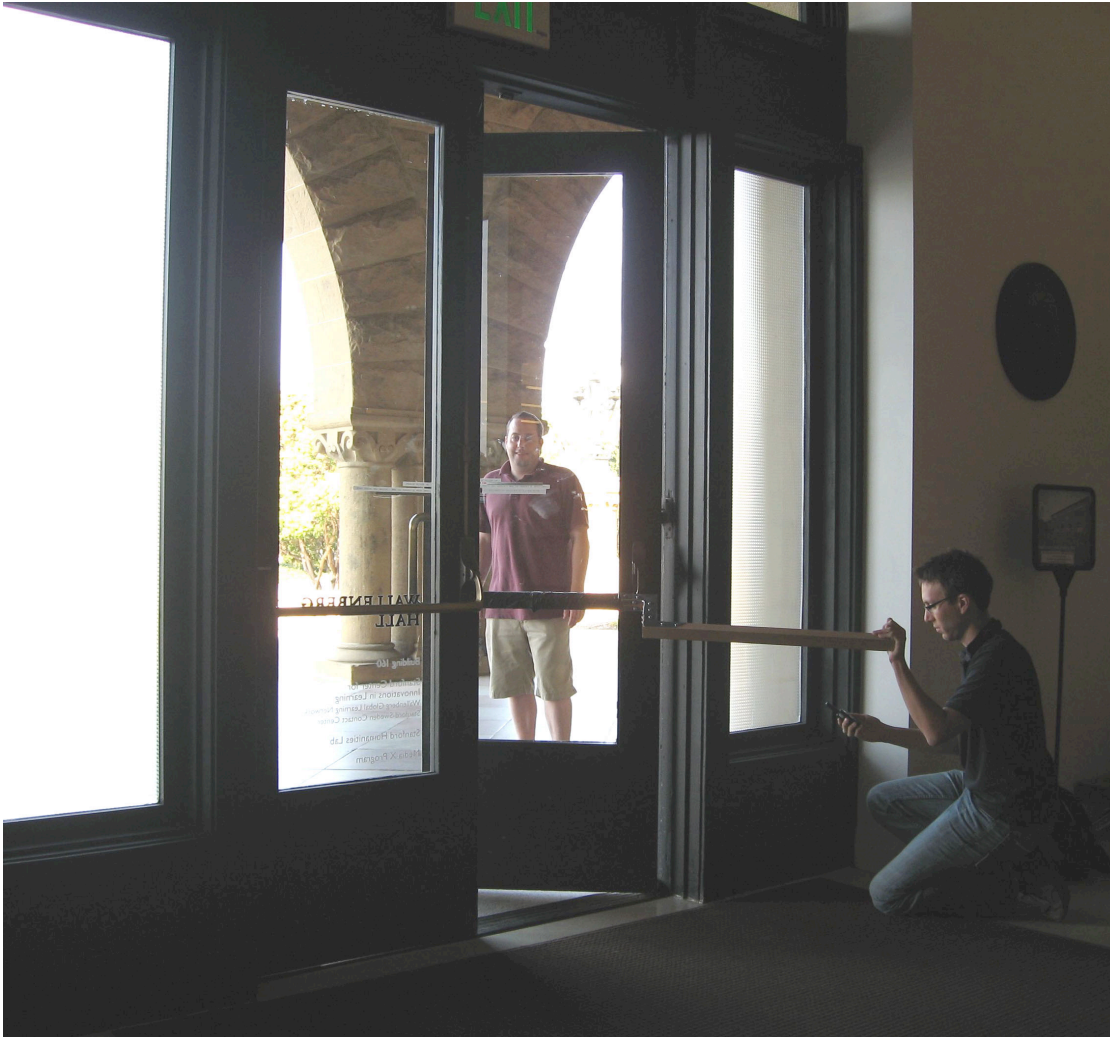
Figure 4. Wizard of Oz setup for gesturing doors study. A hidden door operator uses an armature to gesture the door.
